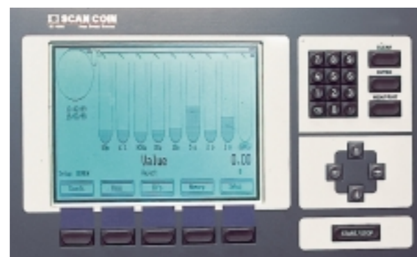
As a bag fills a corresponding column on the display rises.
