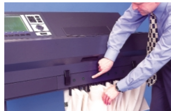
A button illuminates above a bag when it is full. When the bag is changed, pressing the button allows the machine to count coins into the new bag.
