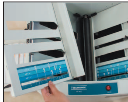
Split table permits removing the top of the fold table for easy maintenance
